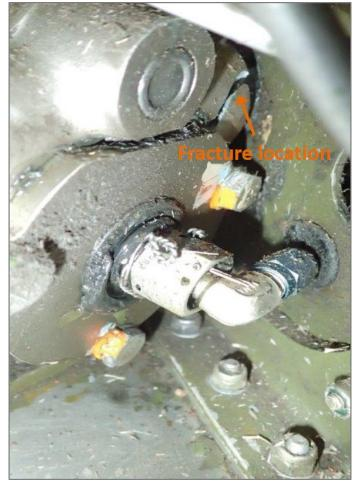
Figure 2: JGA left main landing gear actuator showing the fractured housing
